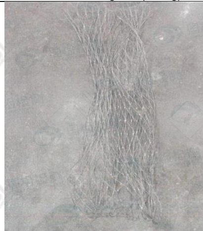
S316L Anti-Fall Safety Net Sample No.:SC202600695 Pressure-bearing test (400kg)
