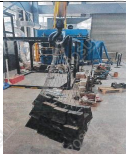
S316L Anti-Fall Safety Net Sample No.:SC202600695 Pressure-bearing test (300kg)
