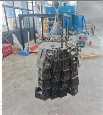
S316L Anti-Fall Safety Net Sample No.:SC202600695 Pressure-bearing test (450kg)
