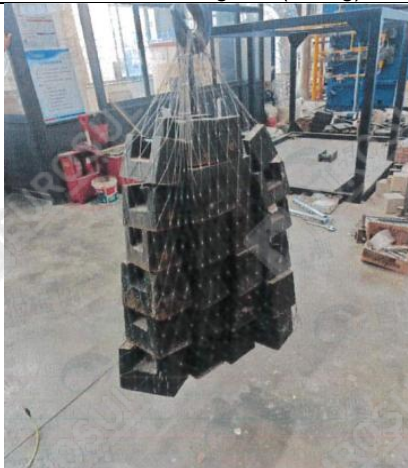
S316L Anti-Fall Safety Net Sample No.:SC202600695 Pressure-bearing test (500kg)
